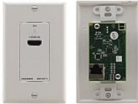
The WP-571 is a PoC DGKat™ wall plate transmitter for HDMI signals. The WP-571 converts an HDMI signal to a DGKat™ twisted pair signal that it transmits to a WP-572
